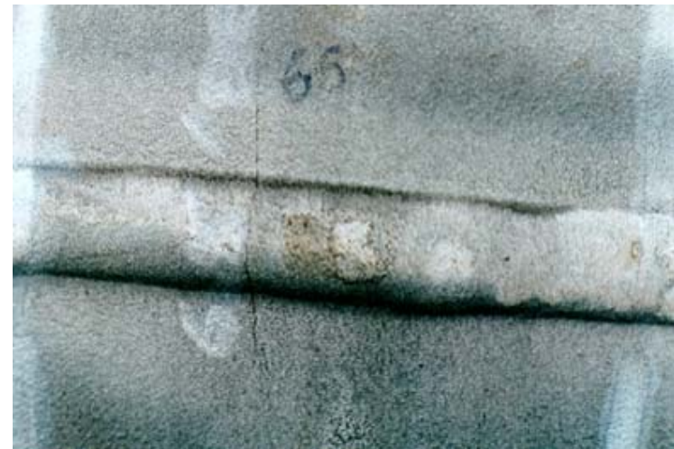
Cricca trasversale in ZF, ZTA e m.b.) (Cricca a freddo – Controllo MT)
